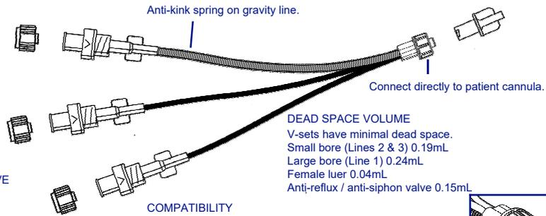
**LINE 2 and 3 (SMALL BORE PE LINED PVC)**
